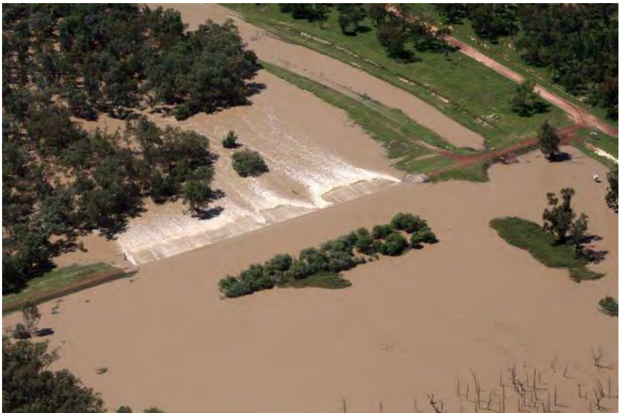
Figure 10 Moolabah Weir – Thuraggi watercourse – damage occurred to the spillway, with movement of concrete slabs, during flooding in 2012
